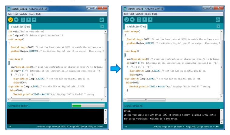
After that, click the "Upload" button to upload the code. Wait a few seconds - you should see the RX and TX leds on the board flashing. If the upload is successful, the message "Done uploading." will appear in the status bar. (Note: If you have an Arduino Mini, NG, or other board, you'll need to physically present the reset button on the board immediately before pressing the upload button.)
