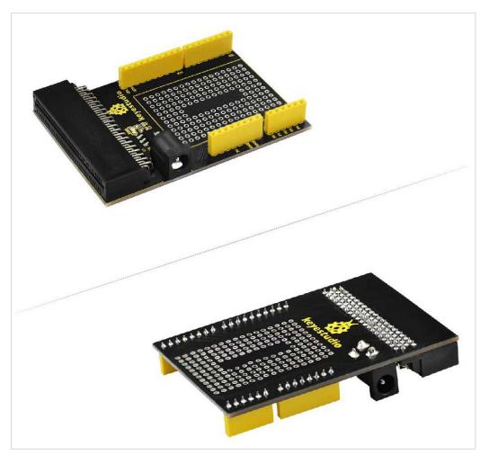
On-board comes with AMS1117 chip, and you can power micro:bit via connecting external jack DC 4.75-12V.
